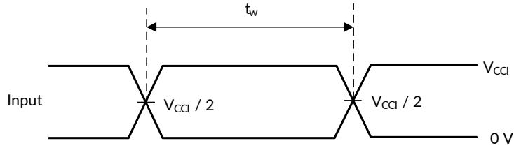
Figure 19. Voltage Waveforms Pulse Duration
